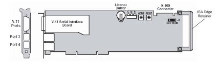
Prepare an SPCI2S or SPCI4 Signaling Board for installation as follows:
